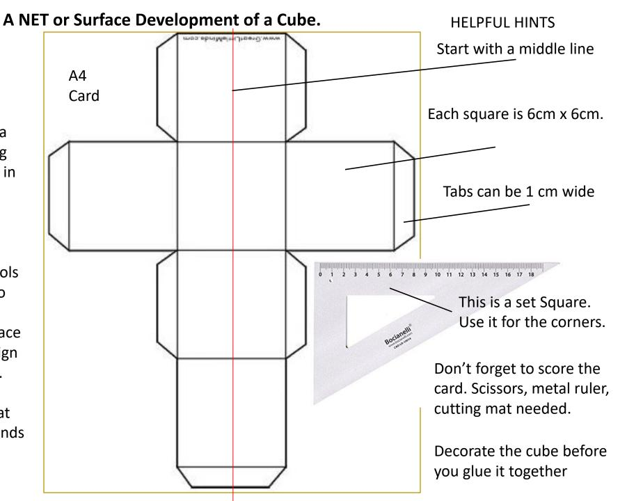
A NET or Surface Development of a Cube. **HELPFUL HINTS** Start with a middle line **A4** Card Each square on the Net is 6cm x 6cm. Tabs can be 1 cm wide 0 1 2 3 4 5 6 7 8 9 10 11 12 13 14 15 16 17 18 Draw all the This is a set Square. symbols on Use it for the corners. the net. Don't forget to score the Your card. Scissors, metal ruler, decorative cutting mat needed. Name design here Decorate the cube before you glue it together
